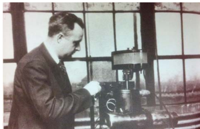
Fig. 1 Midgley with DRL's spark knock investigation engine. At the top is the imaginatively named "Midgley Device"—a kind of periscope for viewing combustion.
